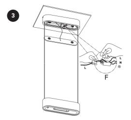
F Connect the power cord and the input line of the lamp body into the terminal according to the identification to fix it
