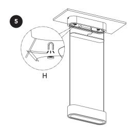
H Then align the decorative cover with the magnet position to fix it, turn on the main power switch
