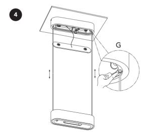
G Press the lifter with your hand to adjust the wire up and down to a suitable position
