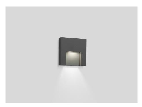
Square wall recessed luminaire made from aluminium; surface Anthracite Grey; powder coated; matt texture; recessed depth 40 mm; suitable for ceiling thickness of min. 12 mm; PCB 3-step binning; light colour 3000 K; degree of protection IP65; PC3; driver not included; light source not replaceable;
